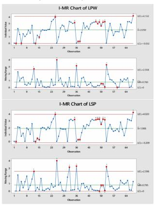
**Figure 6.** I-MR process-behavior charts with logarithmic transformation of two PW point-of-uses in water treatment plant generated using Minitab version 17.1.0)
